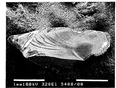
Fig. 5. Irregular piece broken from a crystal of SrTiO 3 used to measure the spectra in Fig. 6.
